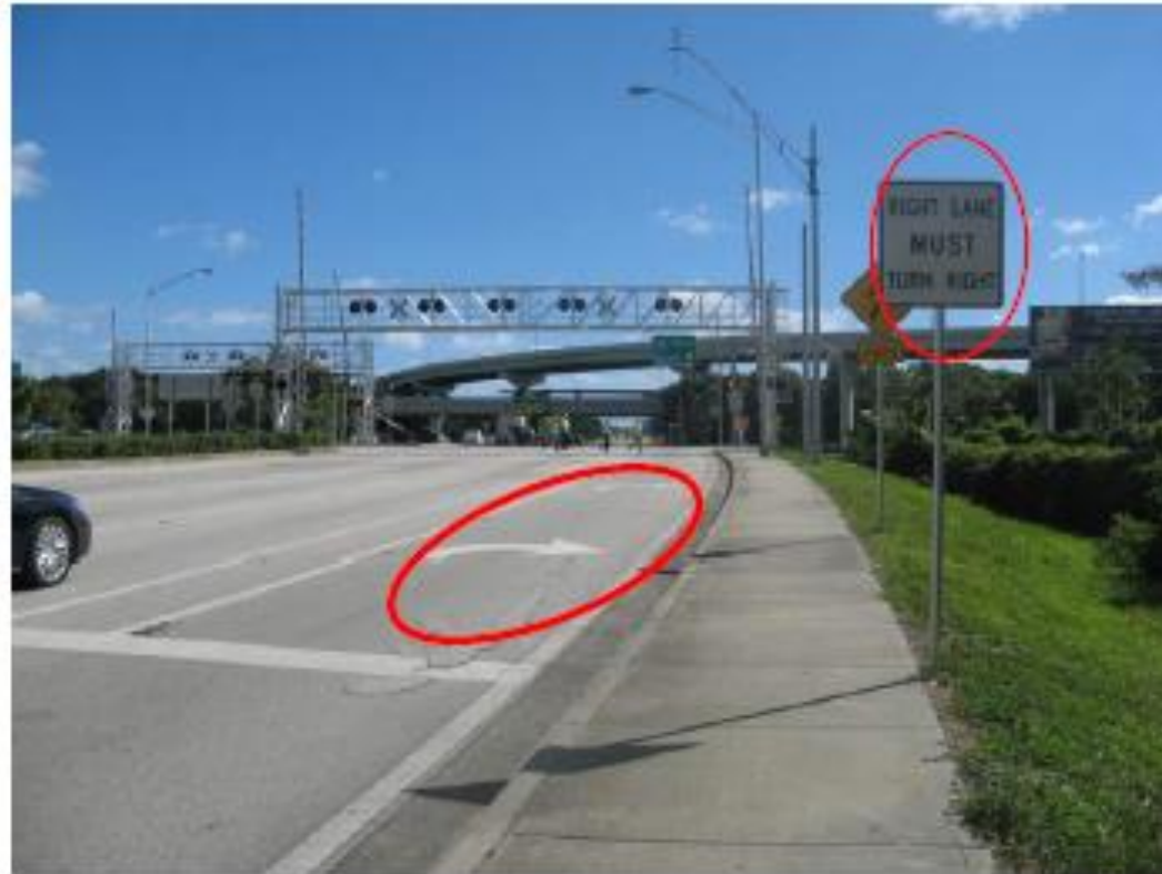
Figure 2 – Example of potentially misleading right-turn sign and pavement markings
