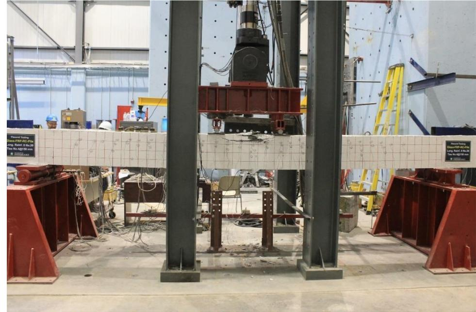
When the applied load was released, the FRP RC beam recovered most of their deflection during the unloading process, because the FRP bars on the tension side did not reach rupture strain; In contrast, the steel specimen retained deflection after unloading
