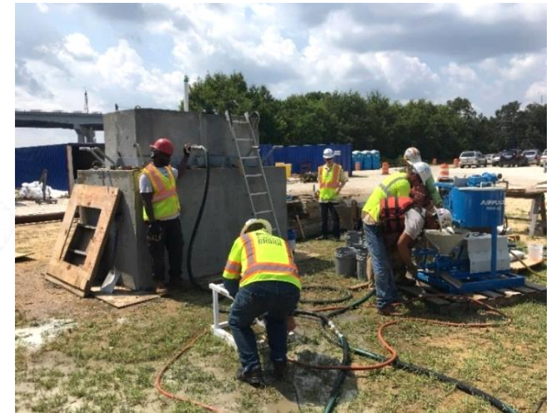
Mock-up testing for the footing to precast column grouted connection. First attempt shown. Three tests performed.
